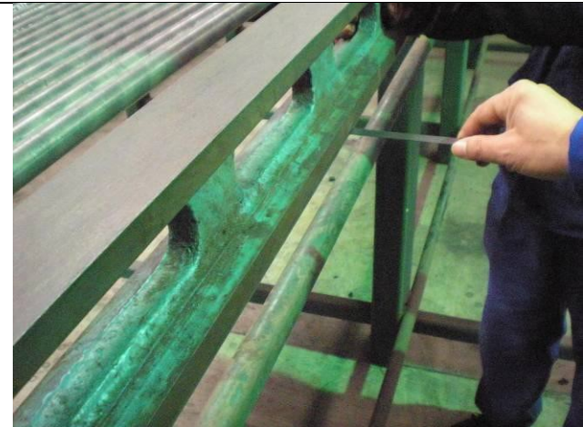
Measuring the straightness
