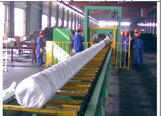
The third wrapping: Polypropylene knitted bag
