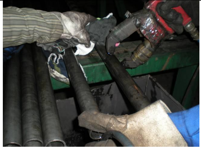
Magnetic Particle Examination
