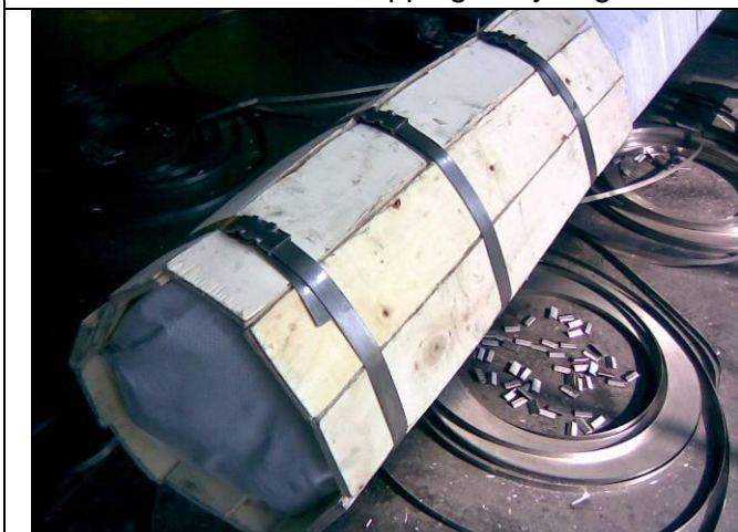
The last wrapping: Batten and metal band
