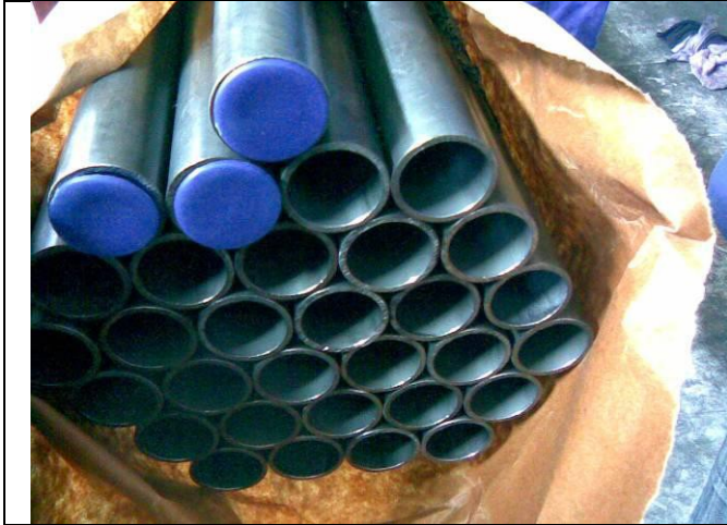
Plugs on tube ends
