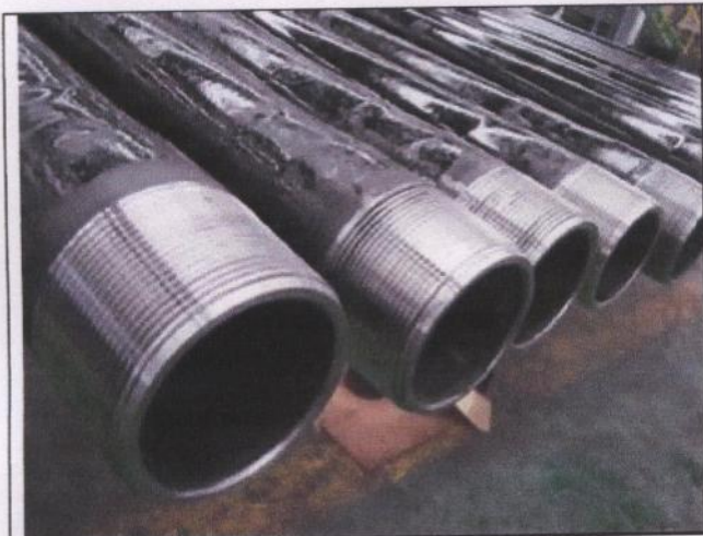
The pipe's end had been machined into screw, one end was male thread.
