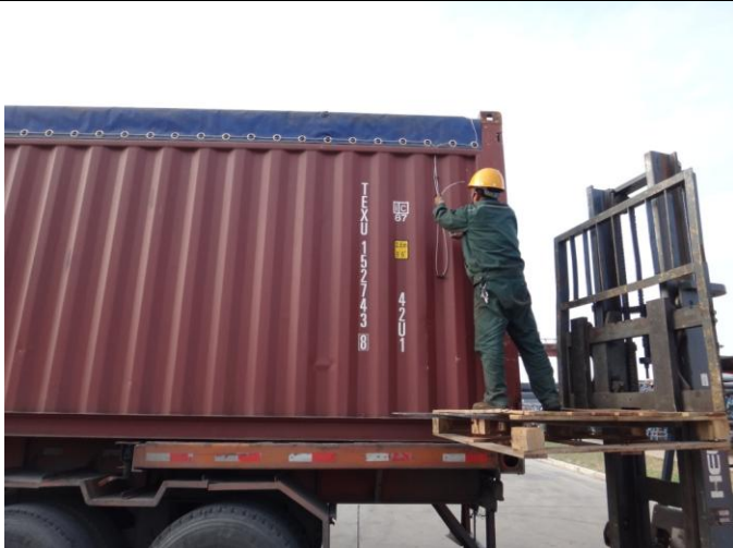
Workers tying up the waterproof tarpaulin
