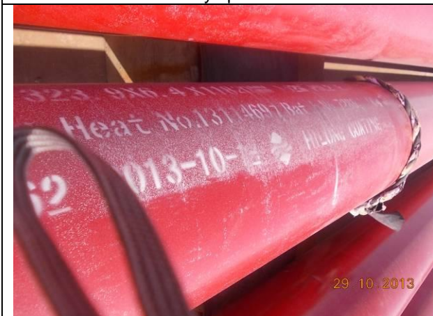
Internal coating were found on the external surface (Atomization)
